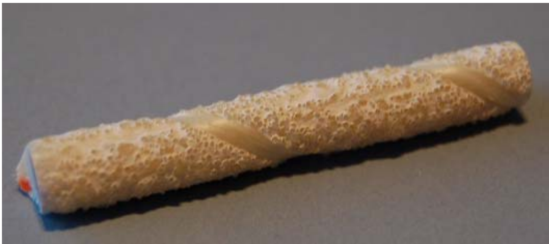
Fig. 1: GFRP composite containing 26 wt% polymer and 74 wt% glass after 1000 hrs of exposure under 70 degrees Celsius.
